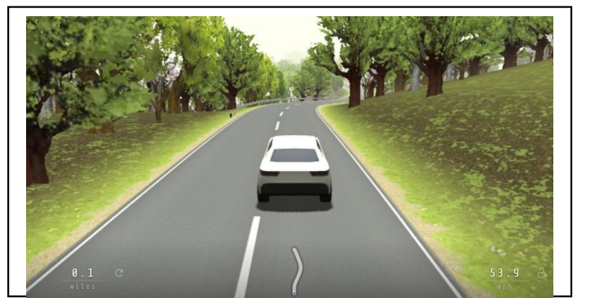
Fig. 7. Forward movement detection resulting in up arrow key emulation in game
