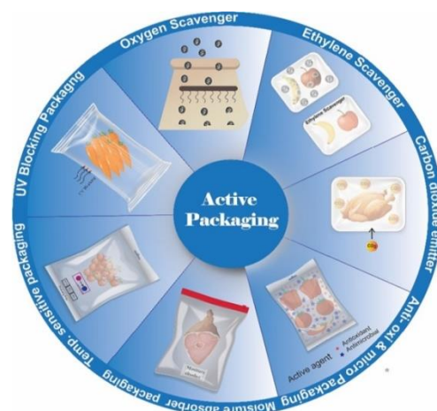
Fig 3: Components of active packaging
